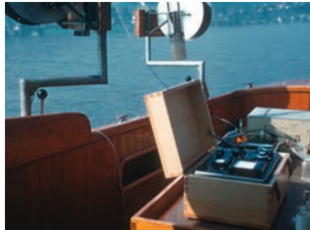
The “oxytester” developed by Heinz Ambühl for measuring oxygen and other values (around 1963).
