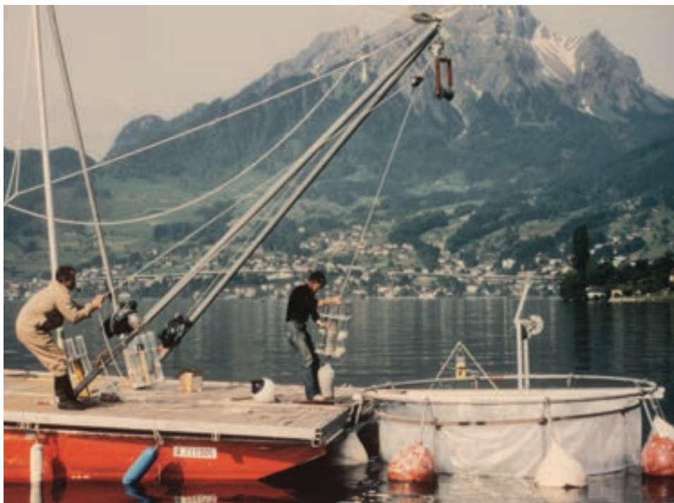
In 1983 the distinct day-night cycles of biological activity of zooplankton in Lake Lucerne were measured in long tubes three metres in diameter.
