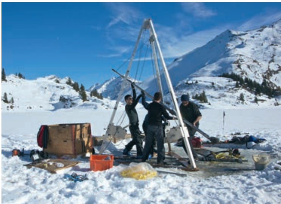
Extraction of a sediment core from the frozen Lake Trüb (canton of Nidwalden). It will be used to reconstruct historic flooding and study the links between particular weather conditions and heavy precipitation.
