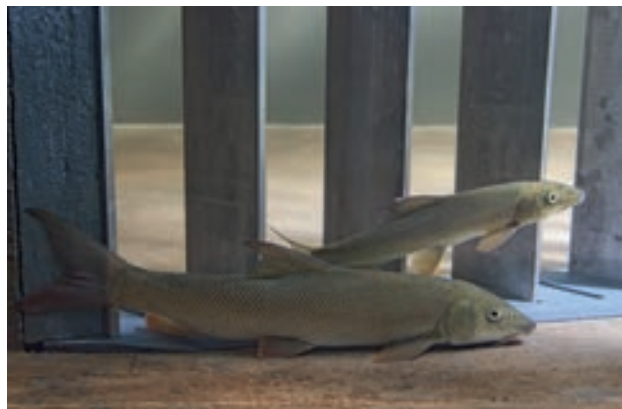
These barbel avoid swimming through the grate and can thus be kept from the dangerous passage through the turbines.
