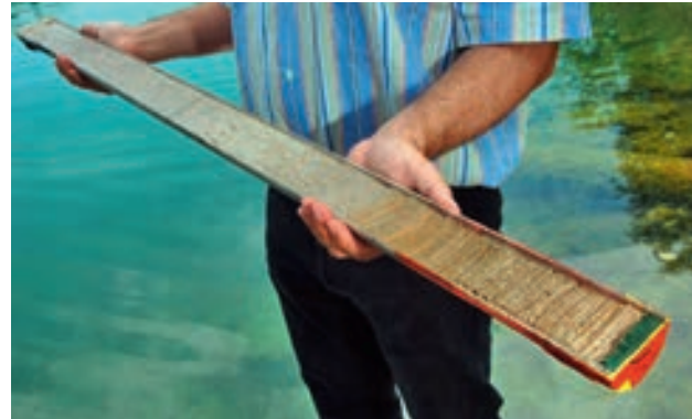
With the help of this sediment core from Lake Greifen (canton of Zurich), Empa and Eawag researchers measured changes in deposits of brominated flame retardants. The annual layers are clearly visible.
