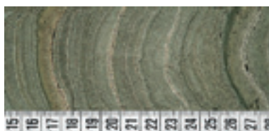
Environmental archive: sediment layers are clearly visible in the split drill core.
