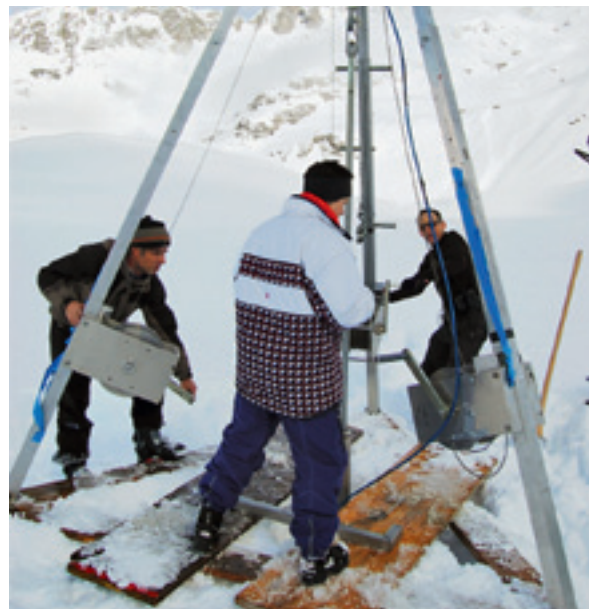
To facilitate core retrieval, the drilling rig is set up on the frozen surface of Lake Stein.
