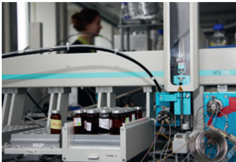
In the lab, wastewater samples are subjected to elaborate chemical analysis.
