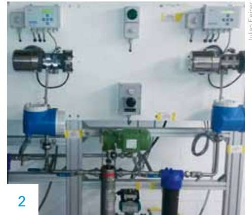
The UV measurement system can be used to optimize ozone dosing for the removal of micropollutants at the Neugut WWTP.
