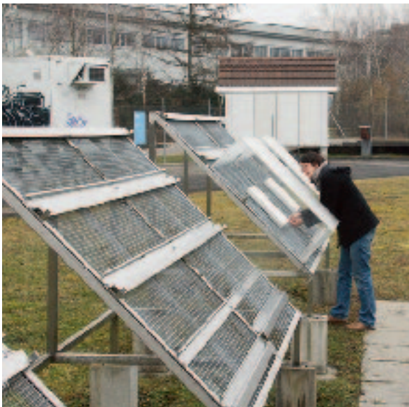
Facade panels with paint containing silver nanoparticles are exposed to rainfall. The rainwater runoff is captured for ecotoxicological assessment, which involves the use of freshwater amphipods ( Gammarus ). In particular, effects on swimming activity and respiration are monitored.
