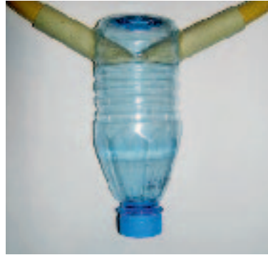
To prevent blockage of the gas line, condensate has to be removed continuously. A proposed simple drain is shown here.
