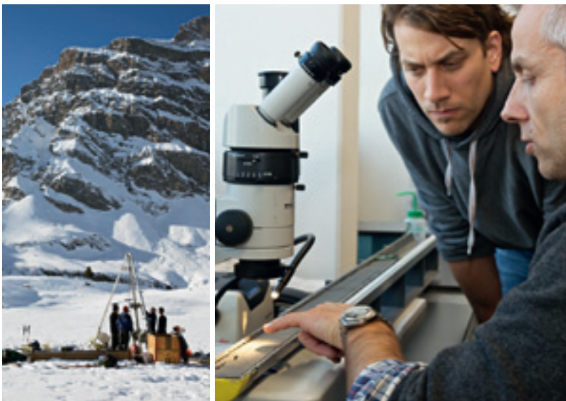
Sediment core drilling on Lake Trüb at the foot of Mount Titlis and analysis of a bisected core.
