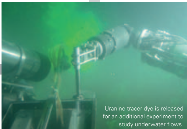
A gripper arm lifts the plastic pipes which are to be driven into the bottom of Lake Geneva.
