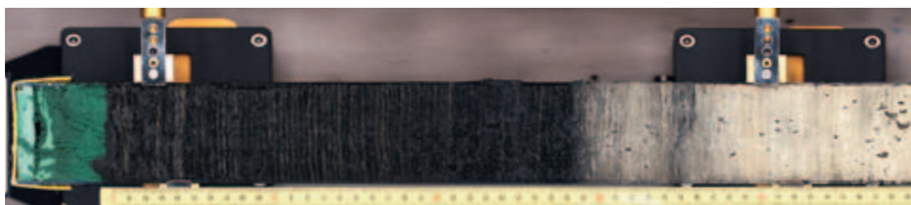
Compounds extracted from a laminated sediment core from Lake Greifen were used to produce a record of historical contamination.
