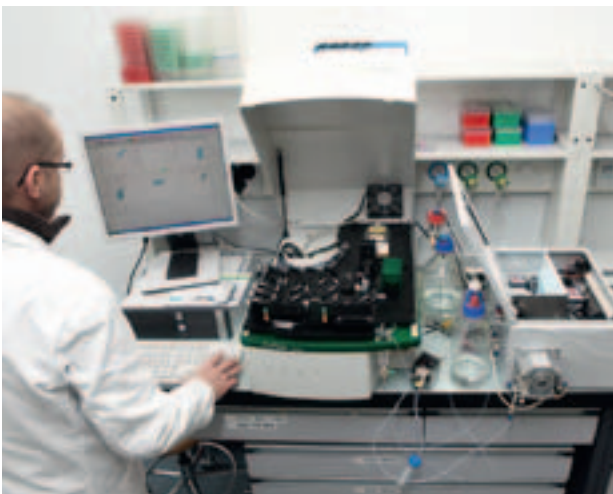
Flow cytometry is used to determine microbial cell concentrations and community composition in water supplies.
