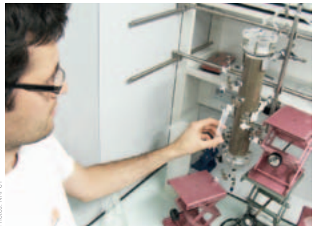
A plexiglas column filled with riverbed sediment provides information on biogeochemical processes during infiltration.
