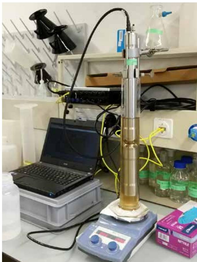
**Figure 15:** A UV-spectrophotometric probe in the laboratory.
