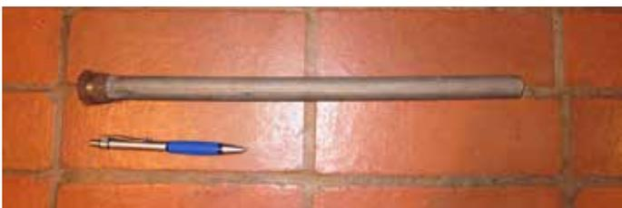
**Figure 14:** Alternatively to adding a dissolved respectively soluble magnesium salt as precipitant, a magnesium electrode can be dissolved-electrochemically.
