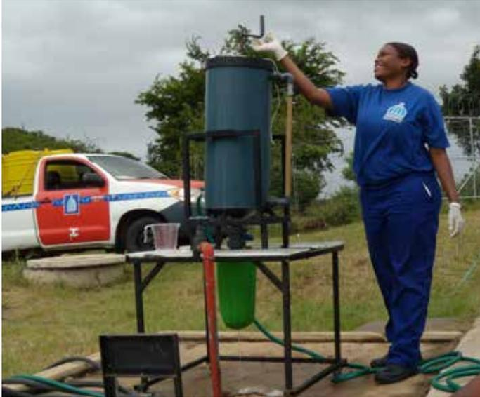
**Figure 12:** The manually operated struvite precipitation reactor produces struvite from urine at the Newlands-Mashu Field Test Site near Durban. The struvite is retained in a filter bag, which is hung beneath the main reactor vessel.
