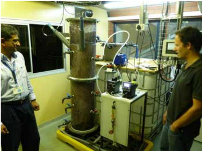
**Figure 7:** The nitrification column at eThekweni's Customer Care Centre sits on a basin to retain spills. A floor drain acts as a back-up for any spills that do not end up in the basin.
