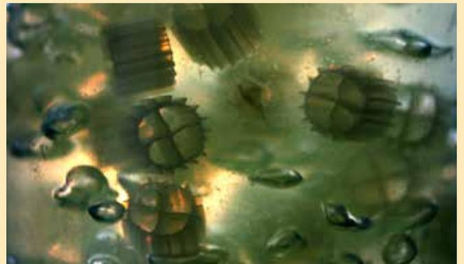
**Figure 2:** Polyethylene biomass carriers provide a large surface for nitrifying bacteria to grow.
