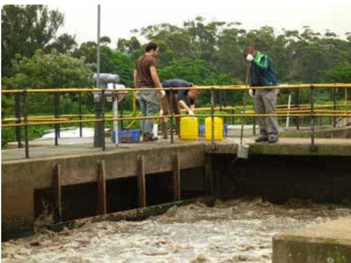
**Figure 8:** A sludge inoculum is taken from the nitrification basin at eThekweni's Norther Treatment Works.
