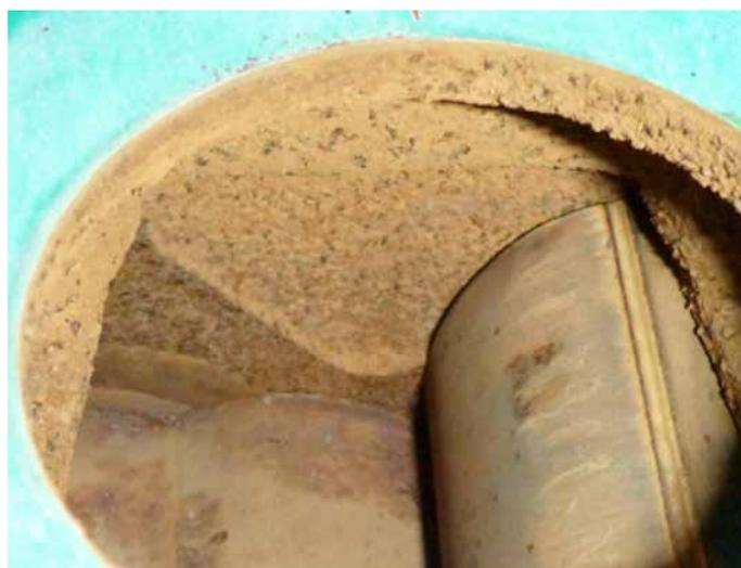
**Figure 9:** The cast steel body of the vacuum pump was the only distiller component susceptible to corrosion.
