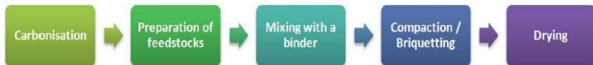
Figure 14: Process chain of charcoal-briquetting (GVEP, 2010)
