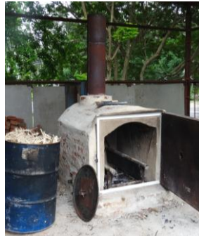
Picture 7: UDSM horizontal drum retort (Ephata, 2014)
