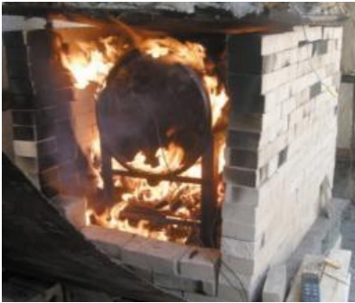
Picture 6: JMU horizontal drum retort kiln (Prins et al., 2011)
