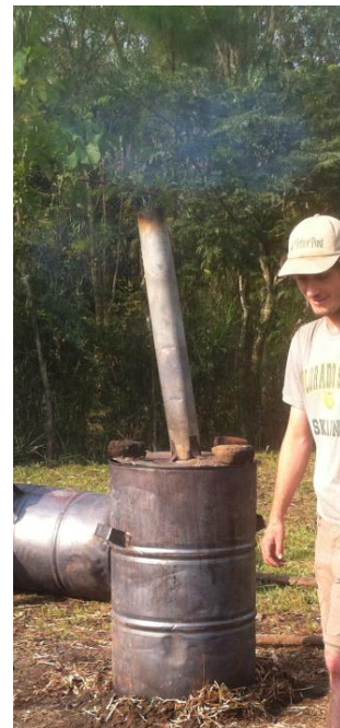
Picture 3: Clear blue smoke from an ARTI-style kiln indicating char combustion (photo: D. Sweeney)
