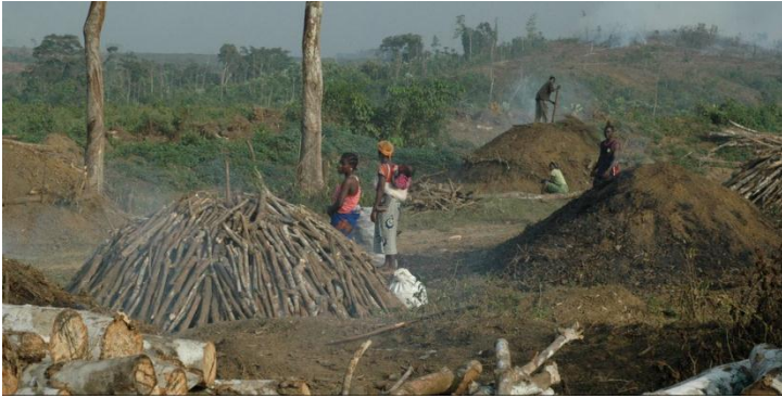
Picture 4: Traditional earth mound charcoal kilns in Liberia (source: BBC, 2012)
