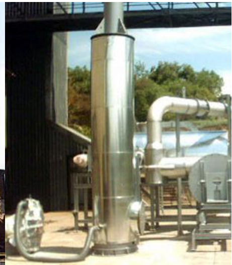
Picture 11: Pro Natura pyrolyzer ( http://www.biochar-international.org/ )
