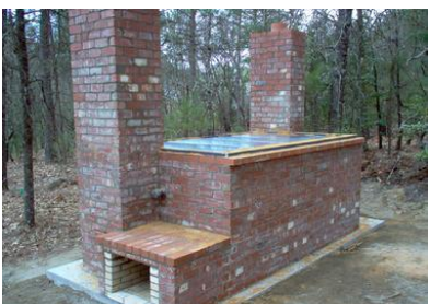
Picture 12: Adam retort ( http://biochar.bioenergylists.org/content/freefarm-adam-retort )
