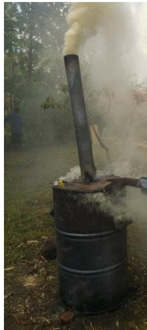
Picture 2: Pyrolysis vapors from an ARTI-style drum kiln (photo: D. Sweeney)
