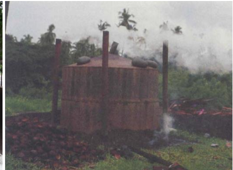
Picture 8: Mark V charcoal kiln (FAO, 1996)
