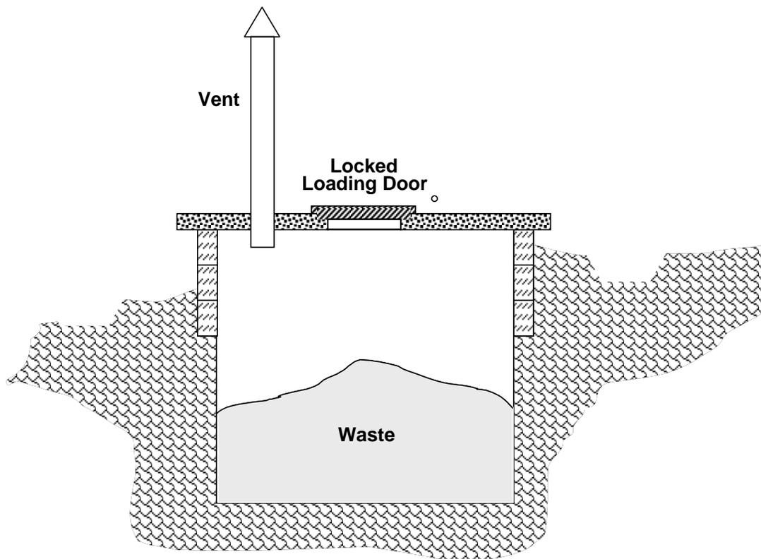
**Figure E2. Cross - Sectional view of secured disposal pit for PHC organic waste**
