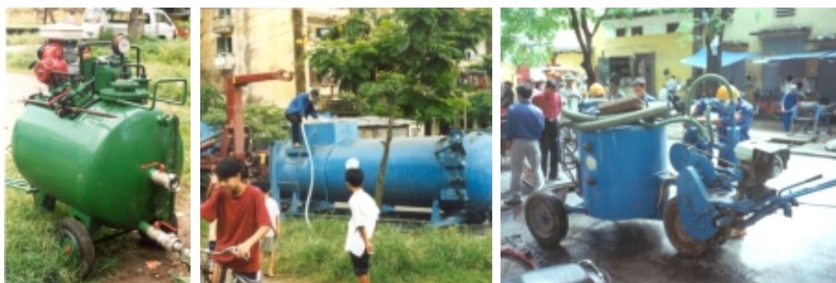
Haiphong made mini-vacuum tug (350 L) for narrow lanes, used together with a intermediate-storage-tank placed in the next accessible road.
