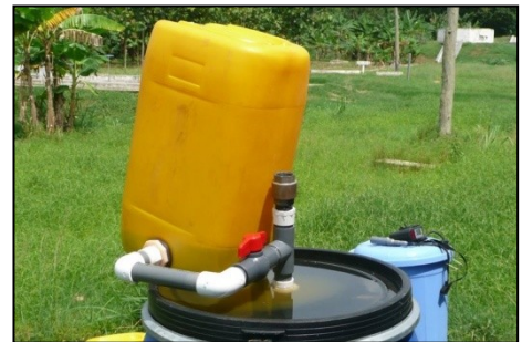
Figure 15: Percolation system made from a 25 litre HD-PE container and 1" PVC pipes, connected to the top hole of the digester
