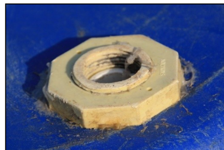
Figure 13: 1" PVC pipe fitting. Allows to connect pipes to the barrel
