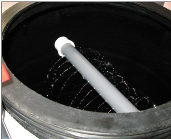
Figure 30: Principle of the percolation system
