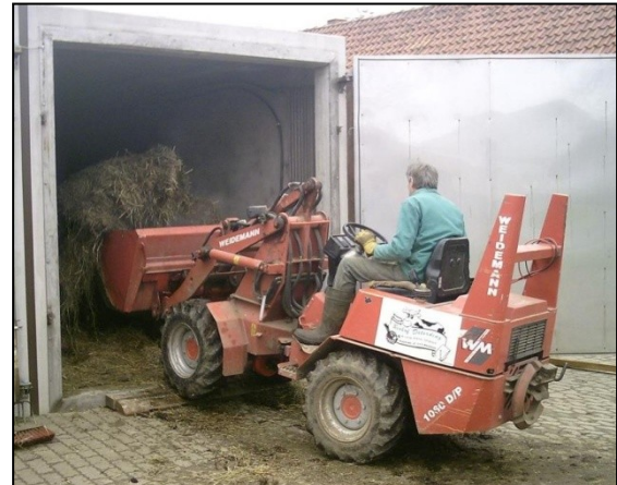
Figure 21: Wheel loader filling a dry digestion garage digester (Stiller 2010).
