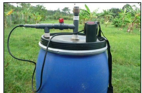
Figure 17: Gas tapping connected to the top hole. Included is the overpressure seal, a PVC valve and the dewatering unit
