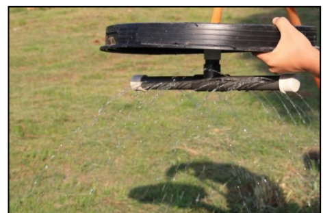
Figure 16: Percolation system connected to the top hole in the lid of the digester
