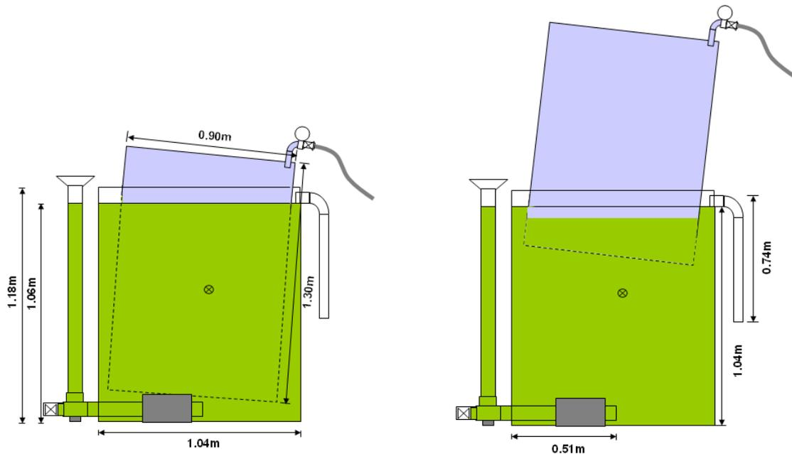
Figure 1. ARTI compact biogas plant scheme (left: with empty gasholder; right: with full gasholder) (Source: Lohri, 2009)
