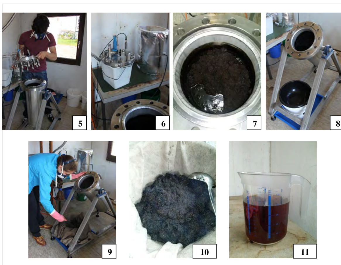
Figure 40: Emptying procedure reactor
