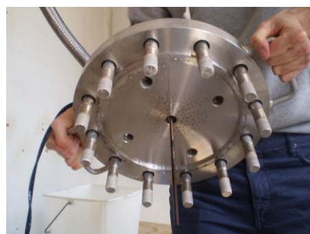
Inferior part of the lid with temperature sensor and screws
