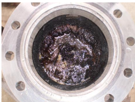
Open reactor (with graphite sealing ring) after a reaction
