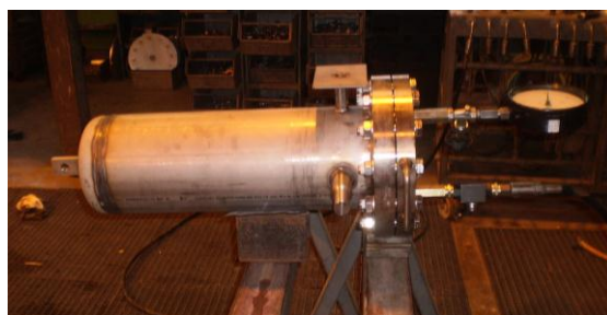
Figure 22: Picture of the reactor during the hydraulic pressure test
