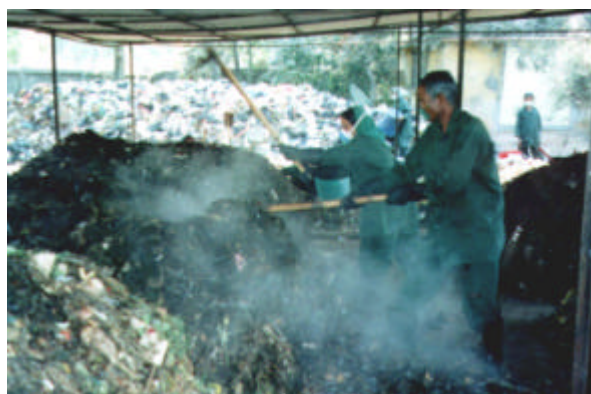
PICTURE 7 TURNING OF DECOMPOSING ORGANIC MATERIAL
