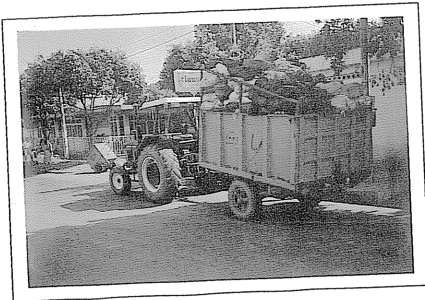
Handcarts of 0.5 m 3 capacity as vehicles for primary collection, trailers of around 6 m 3 payload as intermediate storage units and a tractor for hauling the loaded trailers to the municipal landfill: the case of a small private enterprise in Cucuta (Colombia) serving 50,000 inhabitants. (Photo: SANDEC)
