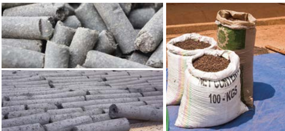
Photo 1: Pellets (top), briquettes (bottom) and crushed fuel produced from FS (right).
