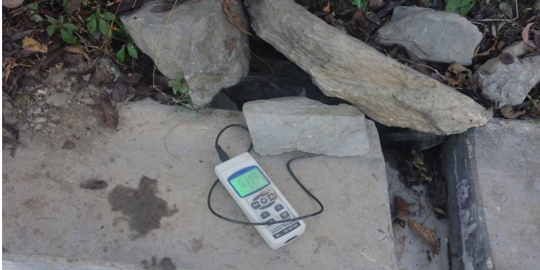
Figure 10 Recording change in electrical conductivity at intake of springs
