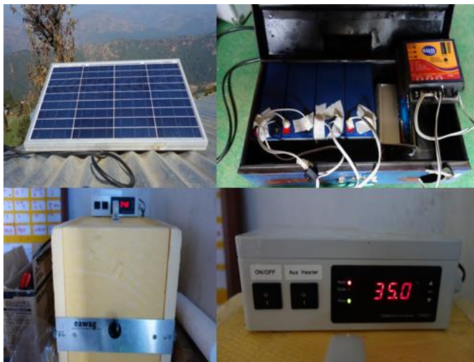
Figure 6 Solar voltaic array, incubator and external temperature regulator box
