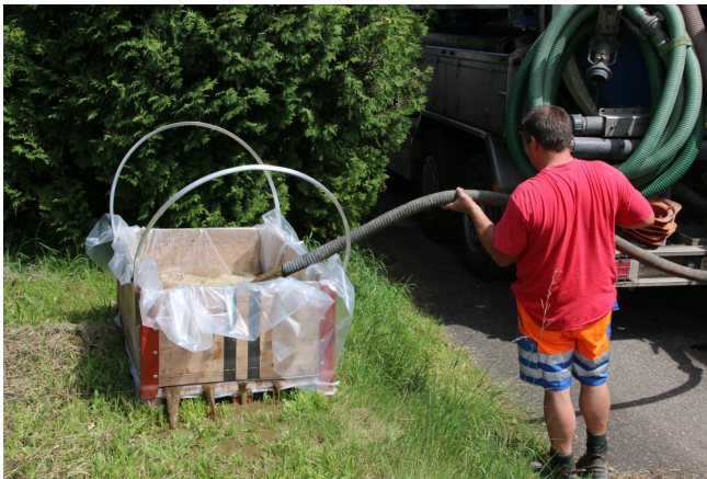
Figure 2: Pilot-scale drying bed
