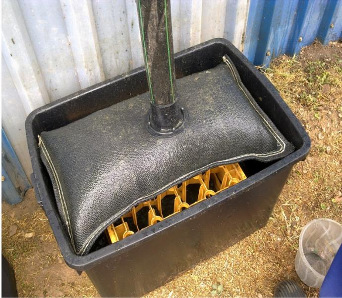
**Figure 4:** Geotextile pillow loaded with FS.
