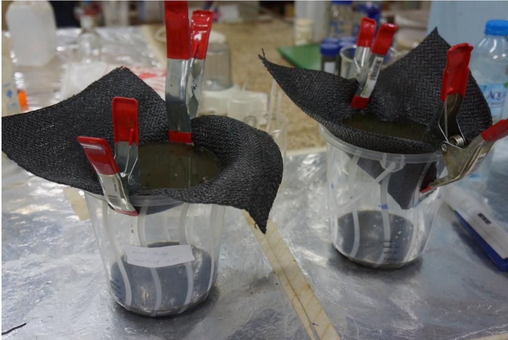
**Figure 1:** Experimental set up of geotextile cone tests
