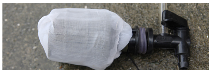
Figure 6: Tap with filter and level tube.
