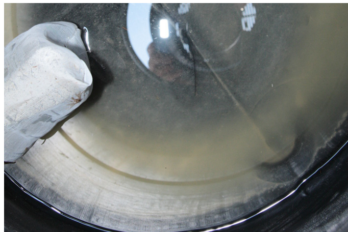
Figure 19: Precipitates in tank 4.
