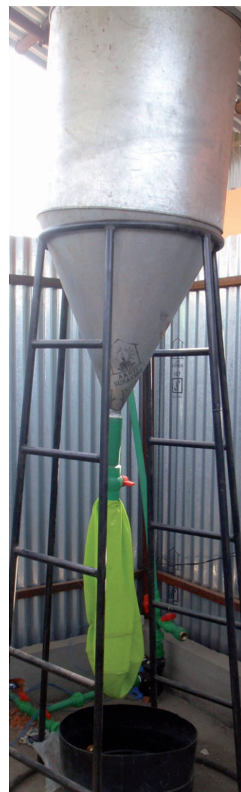
Figure 2: The STUN struvite reactor developed in Nepal.
