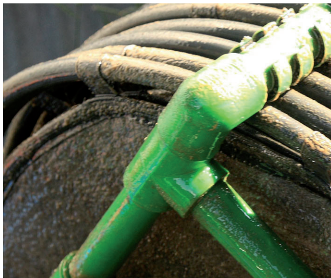
Figure 1: Biofilm growing on the foam coated discs of a RBC.
