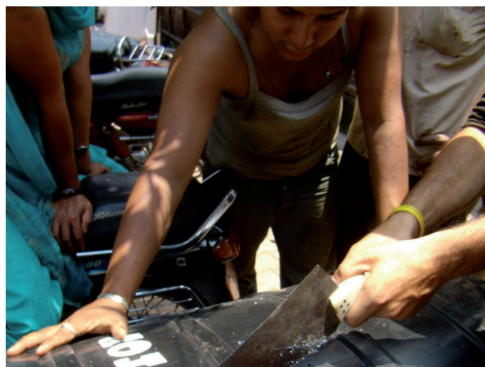
Figure 3: A water tank being cut (top) to produce the reactor vessel (bottom).
