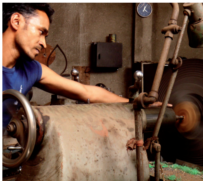
Figure 15: Precise machining of the wooden block holding the nylon bush of the RBC.
