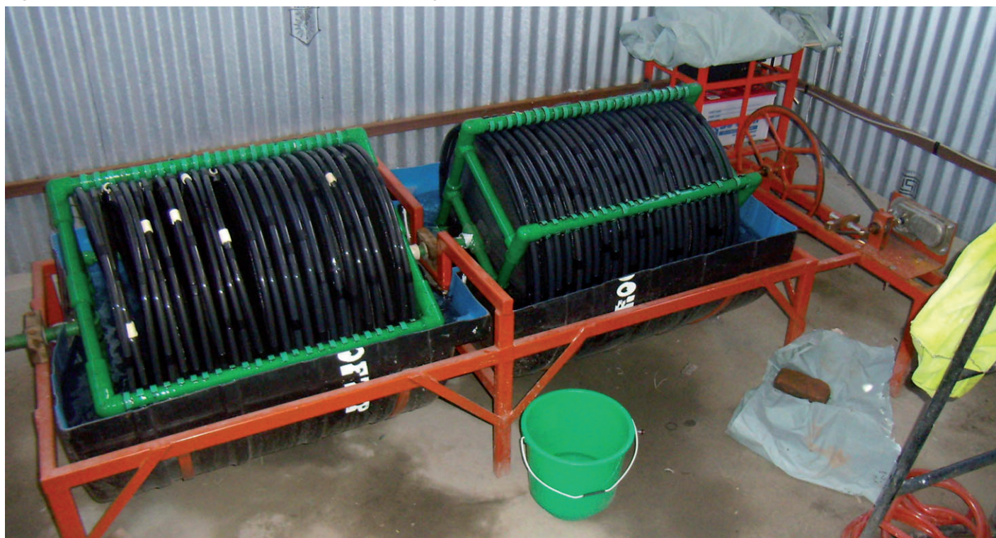
Figure 7: The completed RBC with its drive unit on the right side.
