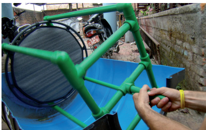
Figure 6: The assembled polypropylene rotor carrying a prototype foam disc is tested in the reactor vessel.
