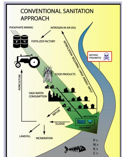
Figure 1: Conventional sanitation approach (source: Morel, A; adapted from Otterpohl R. <http://www.otterwasser.de>)
