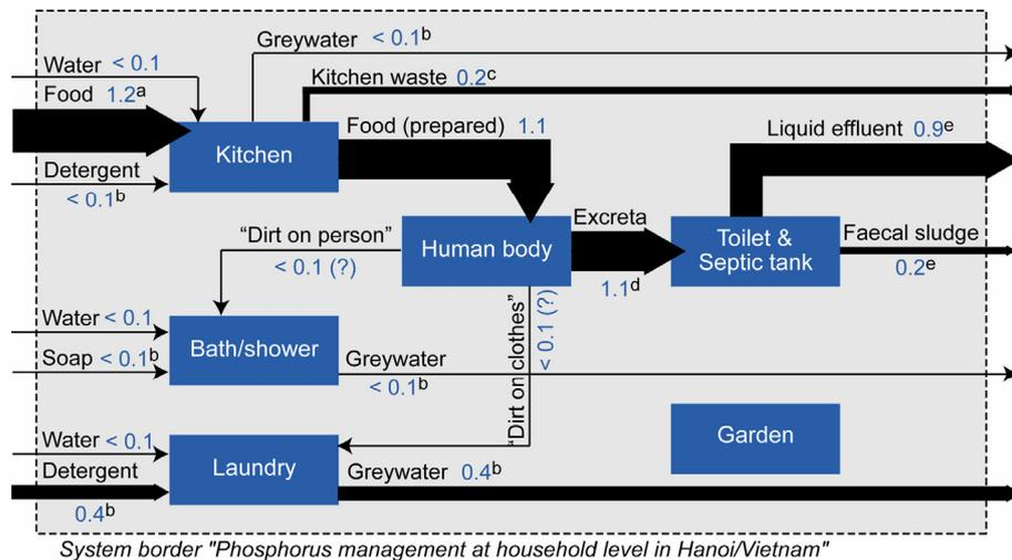
**Figure 4 Average phosphorus flows in urban household in Hanoi.** Flows are expressed in g P cap<sup>-1</sup> day<sup>-1</sup>. Data are based on: <sup>a</sup> FAO (1972), FAOSTAT (2004). <sup>b</sup> Büsser (2006). <sup>c</sup> Diaz et al. (1996), Rytz (2001), Schouw et al. (2002b), Strauss et al. (2003), Sinsupan (2004). <sup>d</sup> Polprasert et al. (1981), Heinss et al. (1998). <sup>e</sup> Montangero and Belevi (2007). Other flows are based on assumptions.
