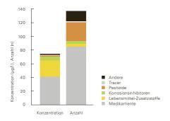
Mean concentrations (left) and numbers of substances (right) in various groups of micropollutants detected in the outlets of eight Swiss wastewater treatment plants (unpublished data from an Eawag wastewater screening study supported by the Federal Office for the Environment).
