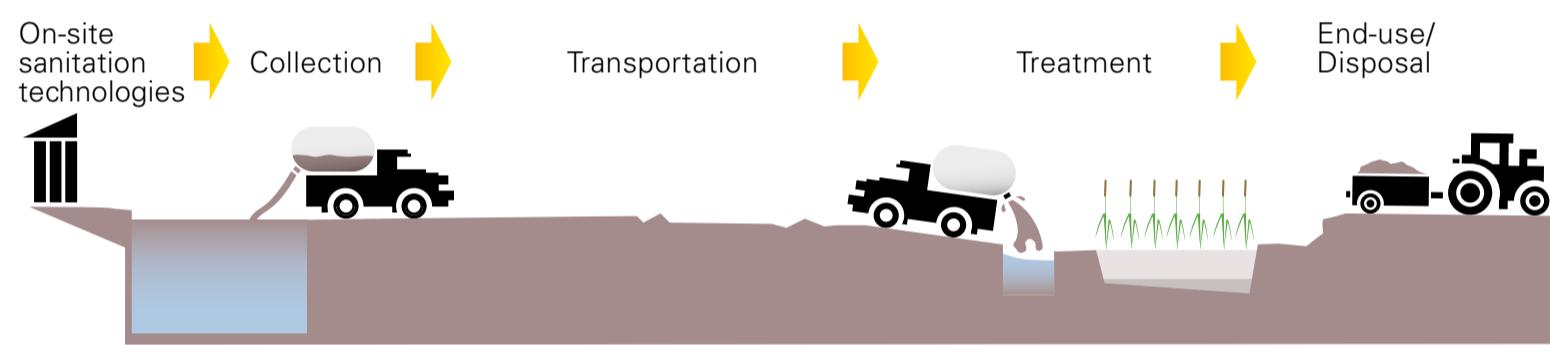
Fig. 2: From collection to end-use or disposal, sustainable sanitation requires a functional faecal sludge management service chain [5].
