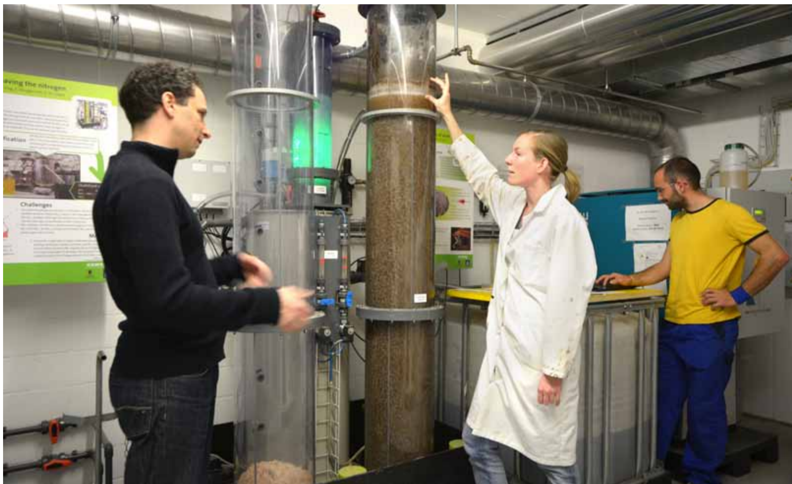
Fig. 1: At the Eawag pilot plant in Dübendorf, urine collected from staff toilets is processed into fertilizers.
