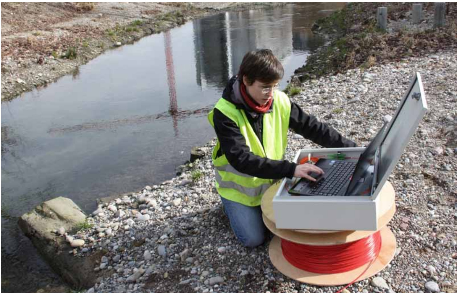
Fig. 1: Anne-Marie Kurth at the field site on the restored Chriesbach stream (Canton Zurich): in the method developed by the Eawag researcher, a fibre-optic cable buried in the streambed is used for temperature measurement.
