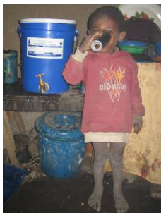
Simple, but effective: bone char filters, as used in Ethiopia, can remove fluoride from drinking water. Eawag researchers are investigating, for example, how the lifetime of these filters can be extended.
