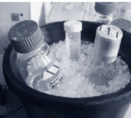
Bacterial cells of the light producing biosensor must always be kept on ice.
