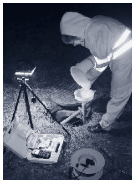
Exfiltration experiment: addition of NaCl solution as a reference signal.
