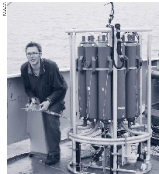
To obtain the water samples we used a rosette sampler with 12 sampling bottles which could be closed off at different depths by a signal from the ship.
