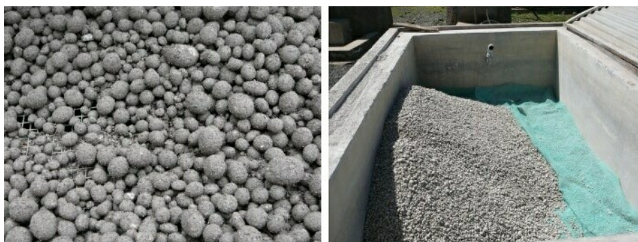
Fig. 7.9 Calcium phosphate pellets that are used in combination with bone char in fluoride removal filters (“Nakuru Technique”)
