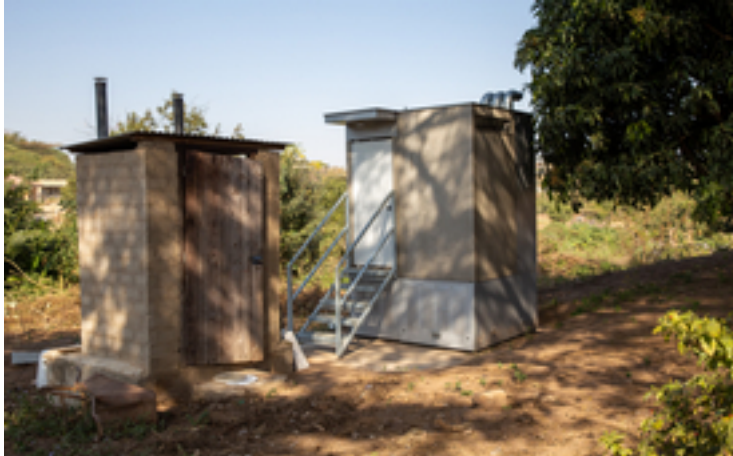
The “Autarky” toilet developed at Eawag (right), shown here in a field test in Durban, South Africa next to a dry toilet. Autarky treats the three separate streams - water, urine and faeces - in situ. (Photo: Lucky Lugogwana)
