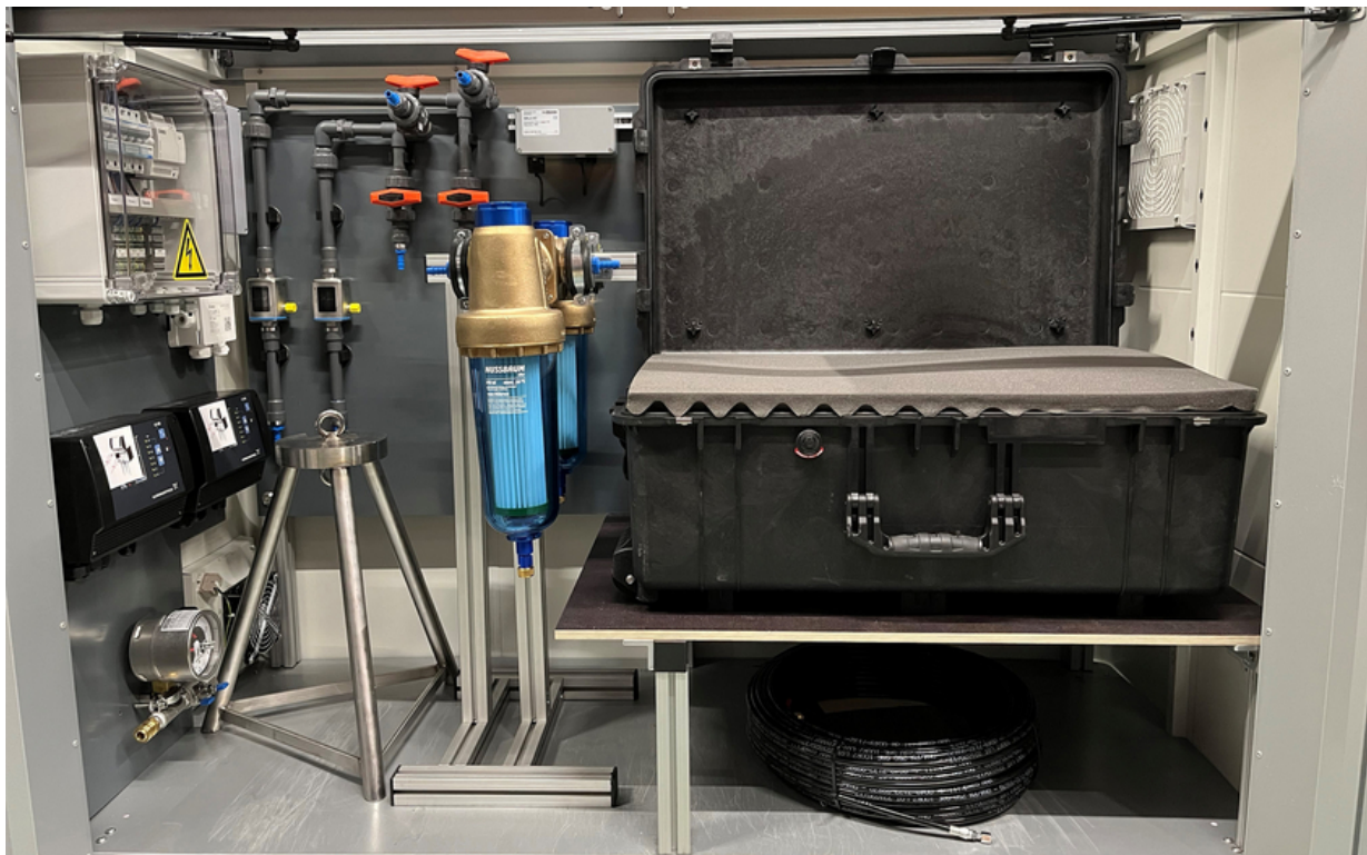
The sensors are located in the box on the surface together with the mass spectrometer (miniRUEDI) (Photo: Eawag, Joaquin Jimenez-Martinez).
