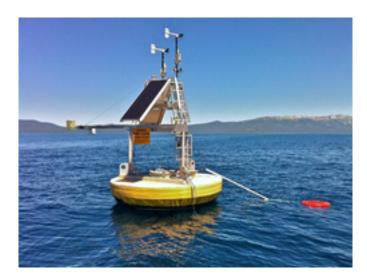
A combination of satellite data and ground measurements, such as from instrumented buoys like this one in Lake Tahoe on the California/Nevada border, were used to provide a comprehensive view of changing lake temperatures worldwide. The buoy measures the water temperature from above and below.
