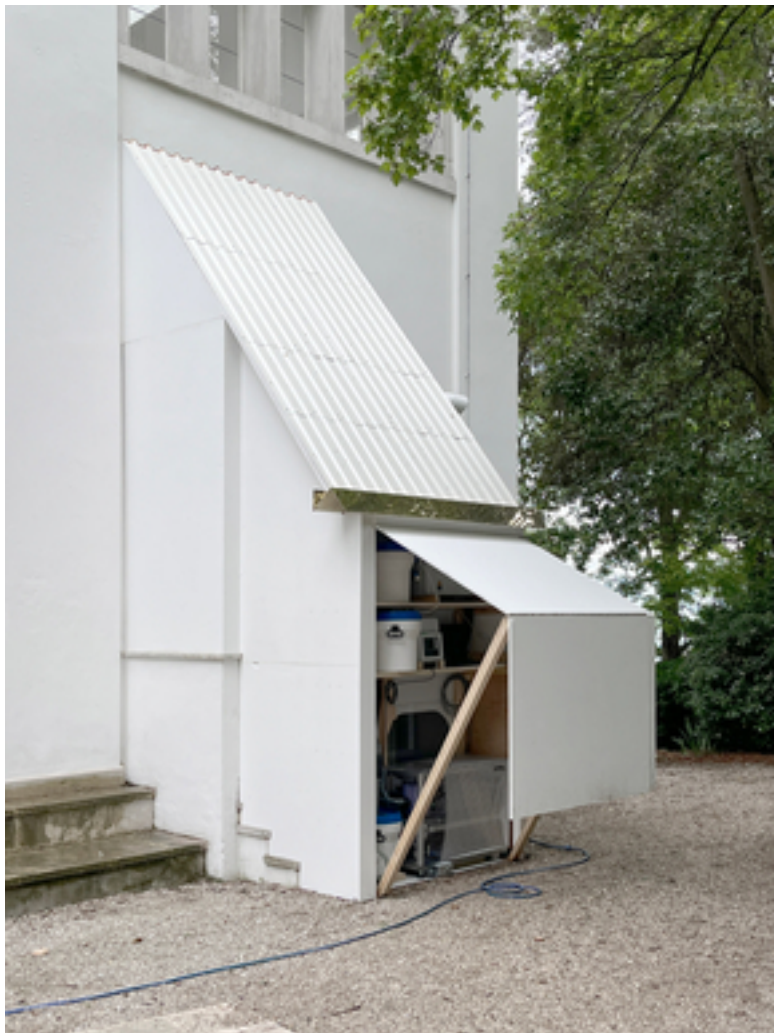
The Nutrient Harvester extracts around 1 kilogram of dry fertiliser from 30 litres of urine. (Photo: ARCH+ SUMMACUMMFEMMER BÜRO JULIANE GREB)
