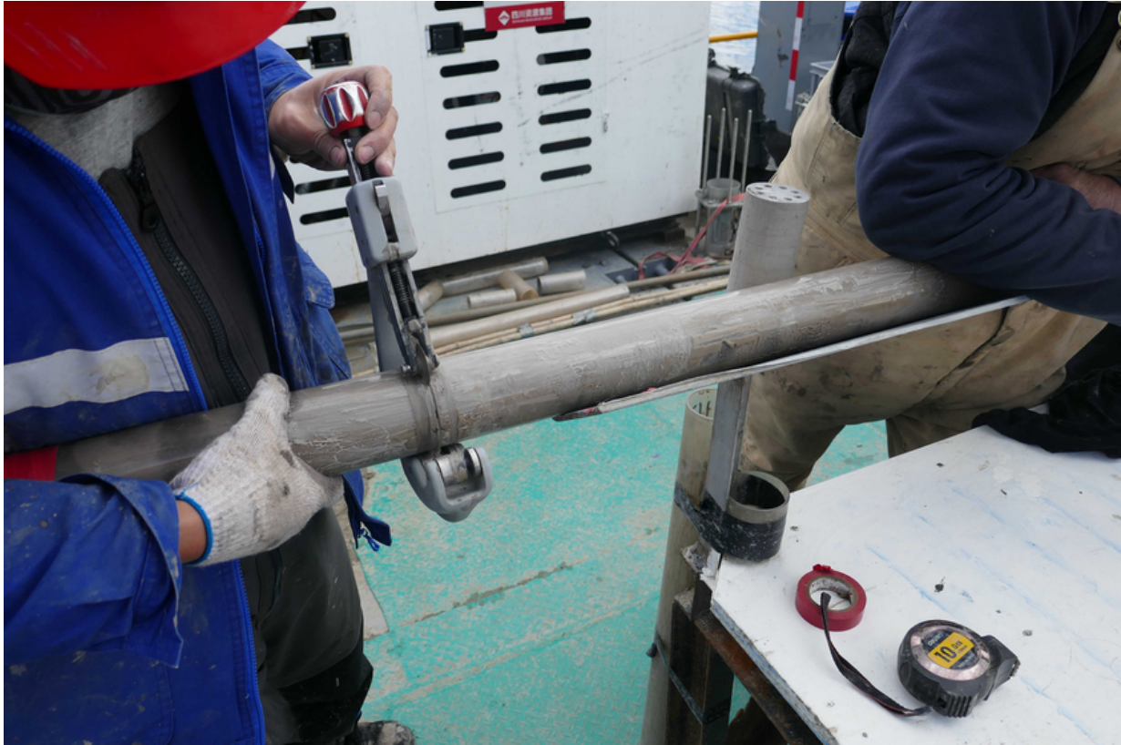
The sediment cores in plastic tubes (liners) are cut into 1-metre-long pieces on the drilling
