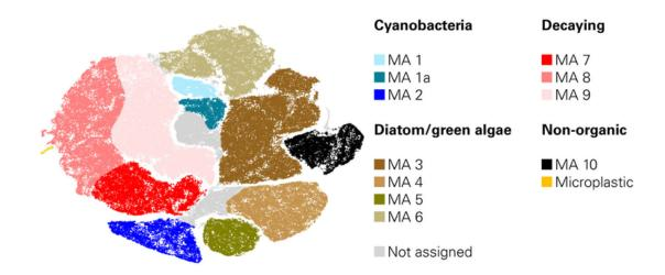
The new method permits analysis of the community structure of biofilms. The various clusters represent subpopulations of cyanobacteria, diatoms/green algae and decaying cells. Individual species, however, cannot always be distinguished. The method can also detect non-organic particles; with assistance from experts at ETH Zurich, some of these particles were identified as microplastics.
