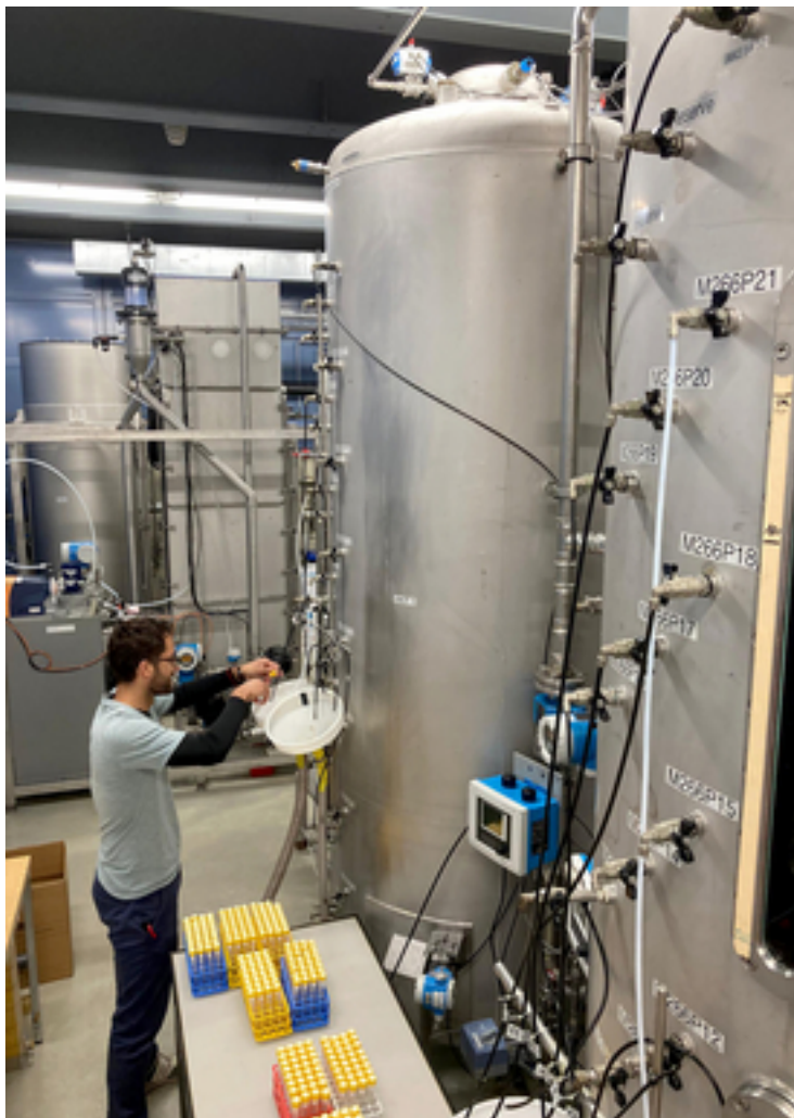
Filtration column at the Eawag laboratory (left) and on the pilot scale at the lake water facility of the Zurich Water Works (WVZ) (right). (Photos: Eawag)
