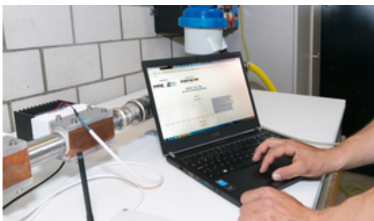
Wireless measurement of the flow in the test assembly. (Foto: Patrick Cipriani / ZHAW)
