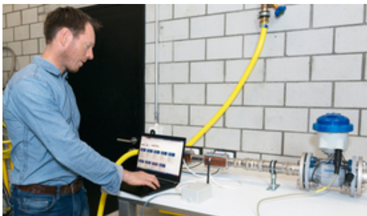
Dr. Frank Blumensaat (Urban Water Management department) uses ADAWIM for wireless measurement of the water flow in the test assembly. (Foto: Patrick Cipriani / ZHAW)
