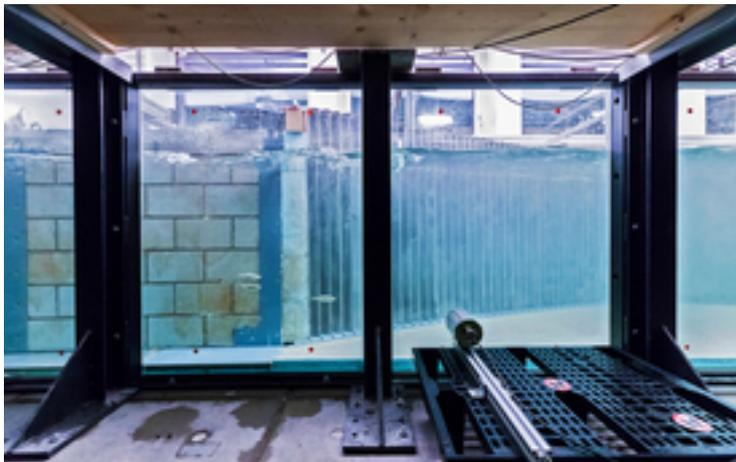
Spirlins in front of the CBR fish guidance screen in the trial installation at VAW. In total, the channel is 30 m long, 1.5 m wide and 1.2 m deep. (Photo: VAW)
