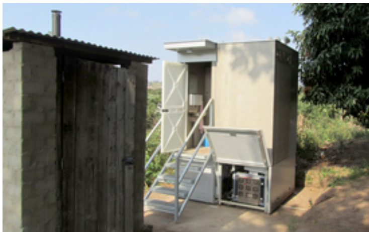
The Blue Diversion Autarky toilet in test on the outskirts of Durban, South Africa. The evaporation module is visible in the front right.
