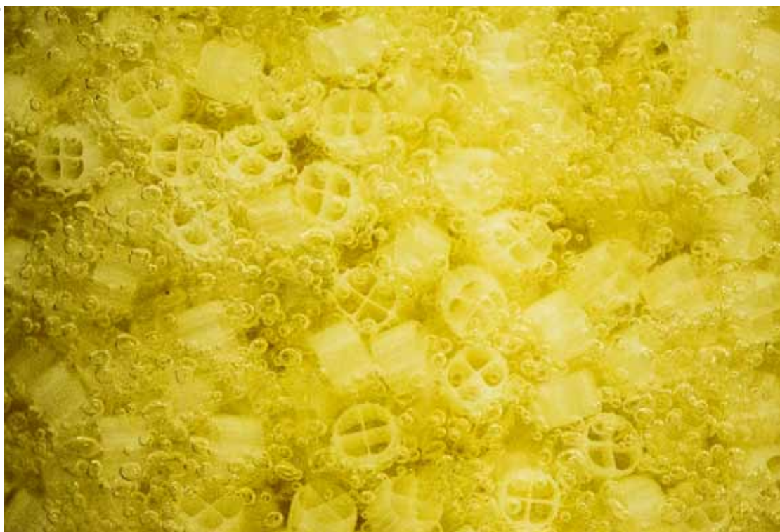
Moving bed bioreactor: plastic biofilm carriers enhance the degradation of organic compounds in treated wastewater.
