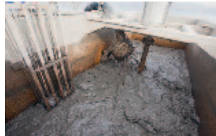
On the pontoon the sludge empties into a buffer tank and is then pumped ashore for treatment.
