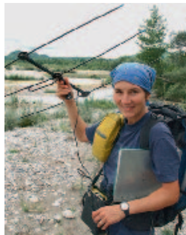
With a tracking antenna and receiver, the radio-tagged amphibians could be located day and night.
