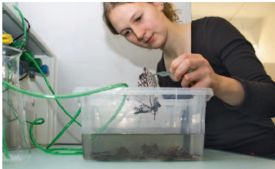
Facade panels with paint containing silver nanoparticles are exposed to rainfall. The rainwater runoff is captured for ecotoxicological assessment, which involves the use of freshwater amphipods ( Gammarus ). In particular, effects on swimming activity and respiration are monitored.
