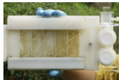
Sample collection: algae on glass slides and two passive samplers used to monitor metals in the stream.
