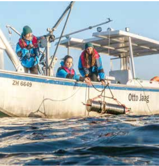
Eawag researchers sink the Aquascope in Lake Greiffen, to capture the underwater life.
