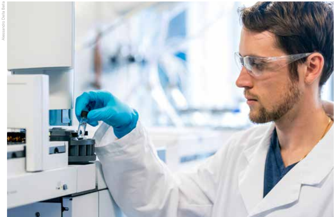
Selective and sensitive analysis of pyrethroid insecticides using gas chromatography coupled to tandem mass spectrometry. Pictured here: scientific assistant Michael Patrick.
