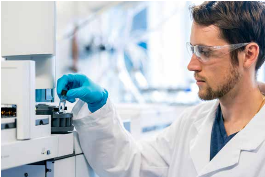
Selective and sensitive analysis of pyrethroid insecticides using gas chromatography coupled to tandem mass spectrometry. Pictured here: scientific assistant Michael Patrick.
