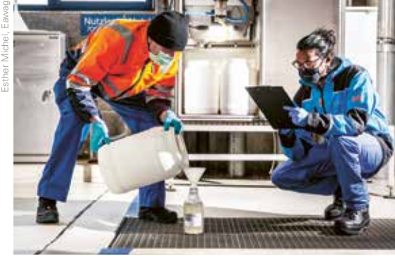
Part of a composite wastewater sample collected at the treatment plant is taken to the lab for analysis.
