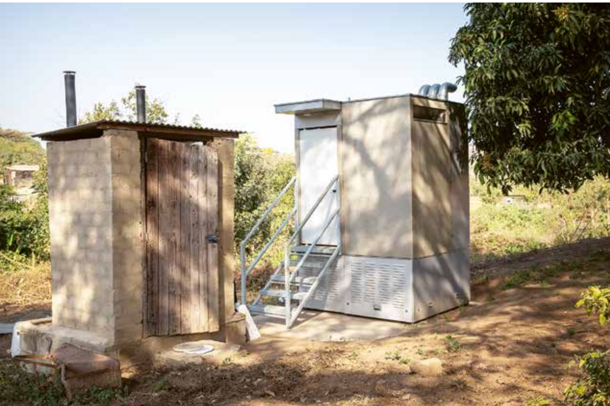
Photo The Blue Diversion Autarky toilet (right) was field-tested in a garden in Durban, beside an existing urine-diverting dry toilet.
