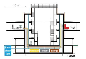
Figure 1. Cross-section of the NEST building indicating the main wastewater flows separated at the source, then collected and treated.
